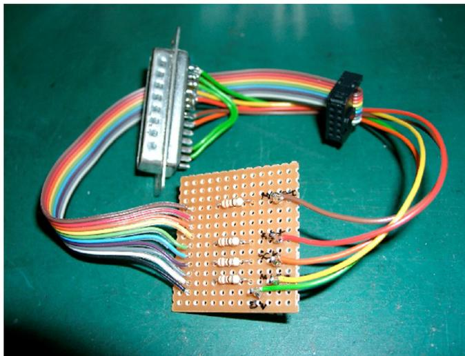
The simple ISP programmer I constructed to use with PonyProg2000
