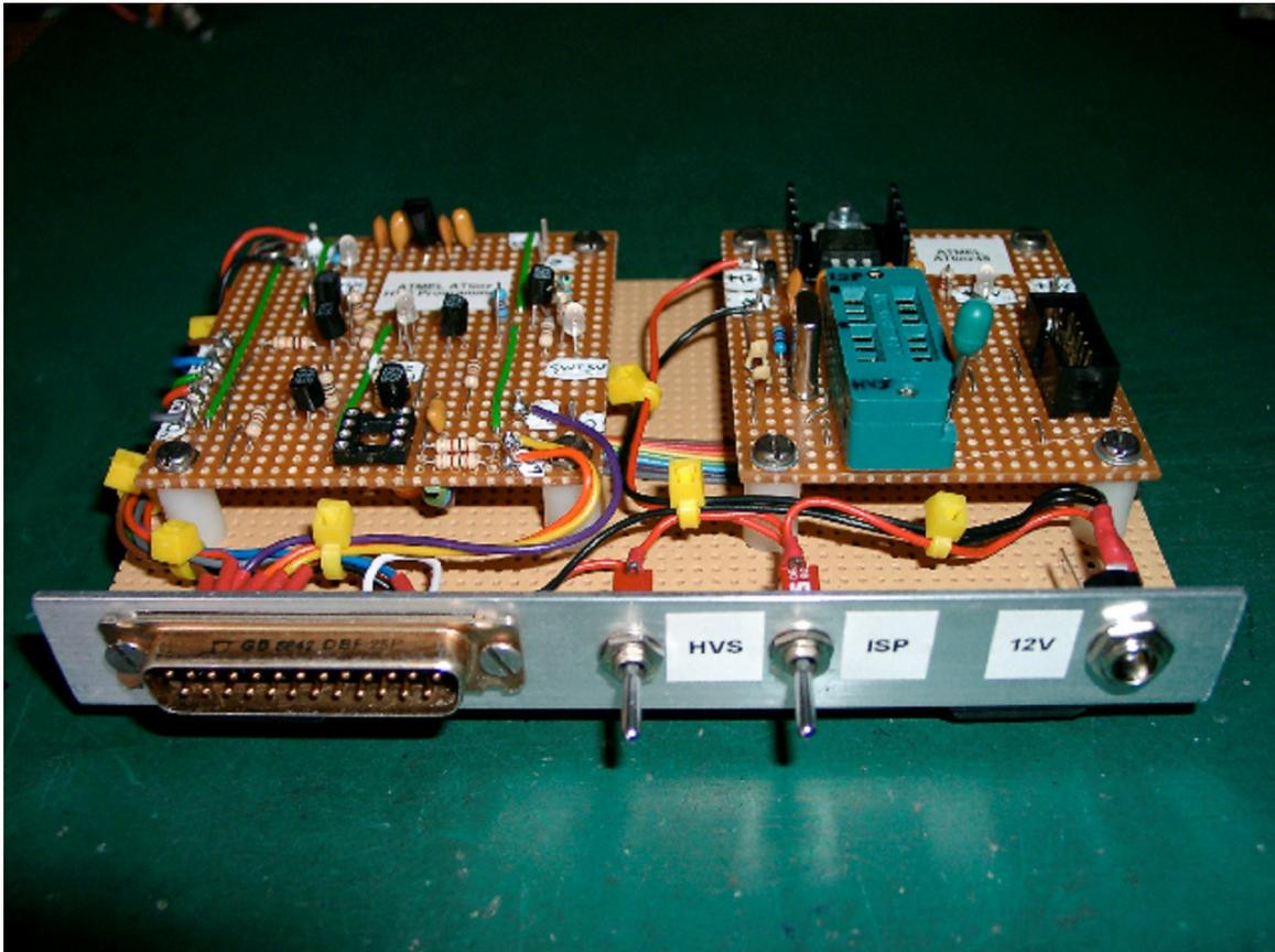
This is the current set up I am using to program the Atmel devices. It is the combination of the two different types of programmers, built on strip board using junk box component.
