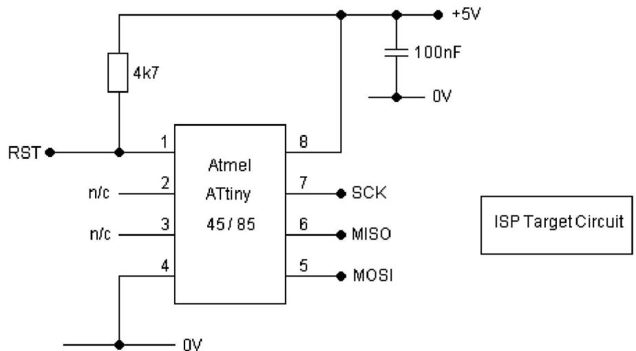
There is one limitation to using ISP programming. The device must either be new and unused or the fuse bits need to be reset to their original state if it has previously been programmed with a version of the SoftRock firmware.
