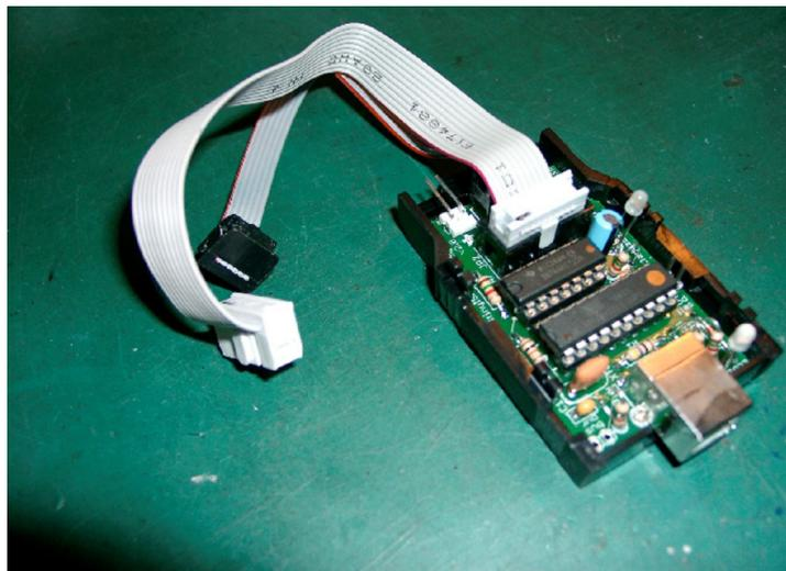
Adafruit USBTinyISP programmer I built from their kit with the top cover removed.
