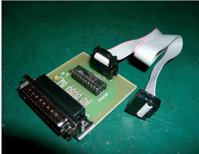
This is an example of a cheap parallel port programmer obtained from a Bulgarian company on ebay that will work with the PonyProg or Avrdude software.
